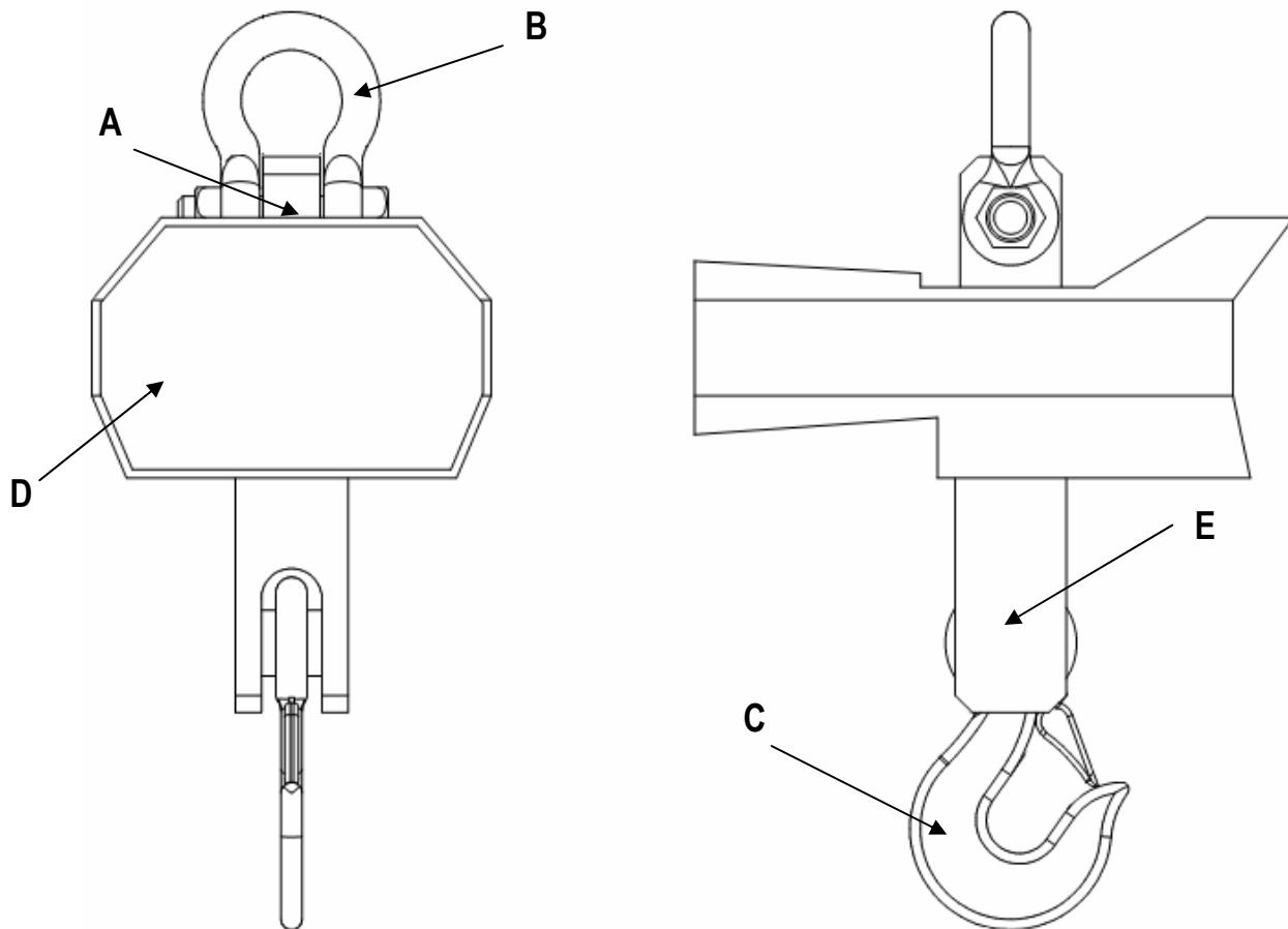
A: body in which there is the tension load cell;
