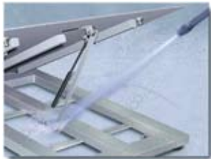
The rugged design incorporates 304 stainless steel construction and four welded-seal load cells with Teflon® cable designed for high temperatures and washdown areas.
